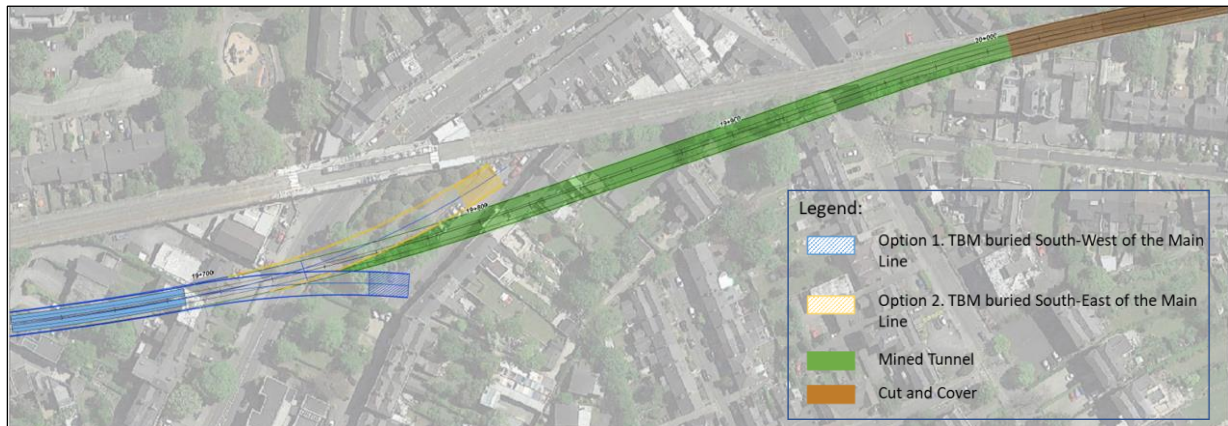
Figure 3-1 Options for TBM Disposal
